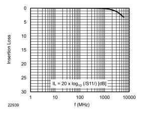
Fig. 6 - Typical Insertion Loss (IL) vs. Frequency
