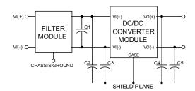
Figure 9. Schematic diagram showing recommended connection of the FLT012A0 filter module with metal-cased DC/DC converter modules.
