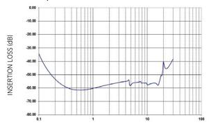
Figure 3: Typical Differential-Mode Insertion Loss in a  $50\Omega$  circuit. (Standard Version, 100MHz Axis max.)
