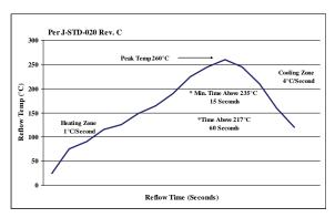
Figure 17. Recommended linear reflow profile using Sn/Ag/Cu solder.
