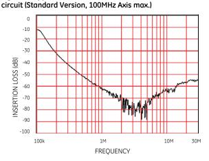
Figure 2: Typical Common-Mode Insertion Loss in a  $50\Omega$  circuit. (-11 Option, 30MHz Axis max.)
