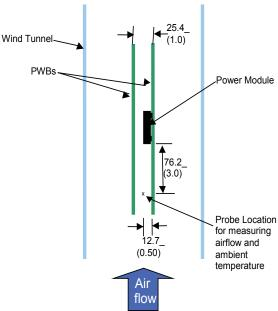
Figure 12. Thermal Test Set-up.
