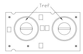
Figure 13. Tref Temperature measurement location.
