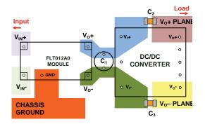
Figure 8. Diagram showing recommended layout of the FLT012A0 filter module with open-frame DC/DC converter modules.
