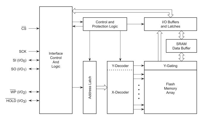
Note: I/O3-0 pin naming convention is used for Dual-I/O and Quad-I/O commands
