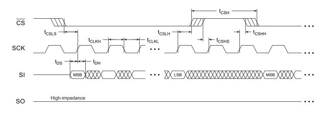
Figure 14-2. Serial Output Timing
